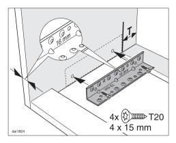
Screw the brackets onto the right and left inside walls of the housing unit as shown. The back edge of the brackets should align with the vertical line drawn up from the front of the spacer strip, and the lower edge aligned with the lower edge of the housing unit side wall.
